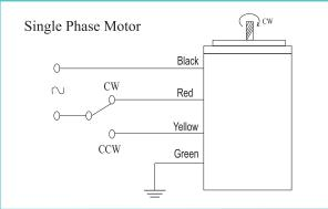
Capacitor is connected internally and is fitted in capacitor cover. Make the connections as shown to rotate the motor in clockwise direction. To Change the direction, flip CW to CCW.
