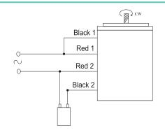
Red wires are for running winding & Black wires are for starting winding. To change the direction, interchange Black wires or Red wires.
