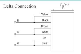
To change the direction, interchange any two wires between U, V & W. For 230 Volt 3 Ph supply, wires are connected as shown.
