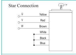
To change the direction, interchange any two wires between U, V & W. For 415 Volt supply, wires are connected as shown. Short White, Black & Blue wire and then insulate properly.
