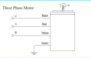
Make the connections as shown to rotate the motor in clockwise direction To change the direction, interchange any two wire between U, V and W.
