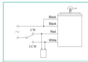
Short Black wires and connect as shown to rotate the motor in clockwise direction To change the direction, flip CW to CCW.
